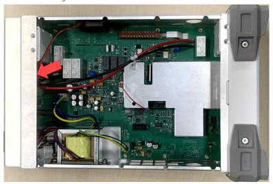
2. Use T10 quincunx screwdriver to remove 4 screws on the middle frame securing the fan, as shown in the following figure.
