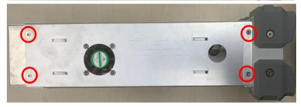
4. Use T10 quincunx screwdriver to remove 4 screws securing the surface board, as shown in the following figure.
