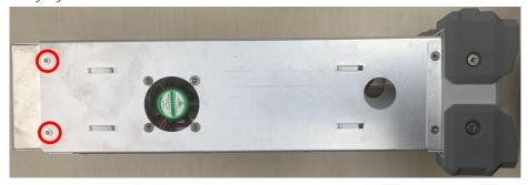
2. Pull out the rear panel by slightly force, as shown in the following figure.
