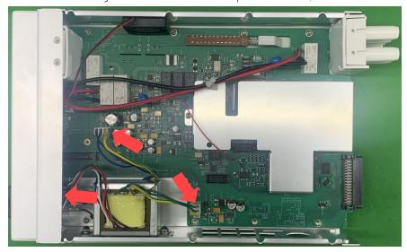
2. Use T10 quincunx screwdriver and needle-nose pliers to remove 2 screws on the middle frame securing the transformer, as shown in the following figure.
