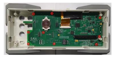
6. The displace screen can only be taken out when the key board is removed, as shown in the following figure.
