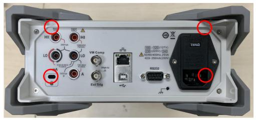
2. Use T10 quincunx screwdriver to remove 2 screws securing the outer frame, as shown in the following figure.
