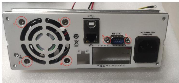
6. Remove 3 screws securing the rear cover, pull out the RS232 wiring interface, as shown in the following figure.
