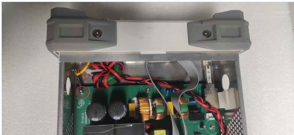
3. Use T10 quincunx screwdriver to remove 4 screws on the edge of front cover, as shown in the following figure.
