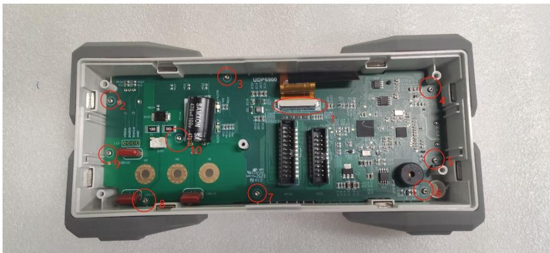
8. Take out the key PCB, button, and screen module to complete the disassembly of front components.
