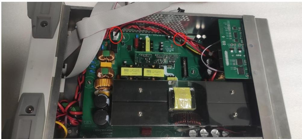
3. Use T10 quincunx screwdriver to remove 4 screws on the edge of rear cover to open it, as shown in the following figure.
