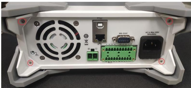
2. Pull out the rear modules by slightly force, as shown in the following figure.
