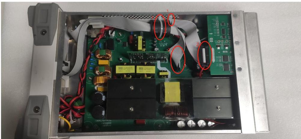
2. Use T10 quincunx screwdriver to remove the grounding screw on the rear panel, pull out the power wire connected to the PCB (the ground wire of UDP6952 and UDP6953 are in the middle of the PCB), as shown in the following figure.
