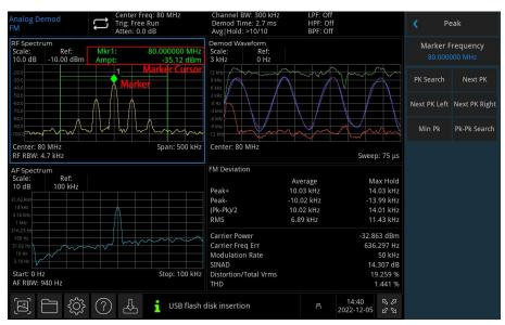
Figure 3-1 Reading of Marker Cursor Reading
