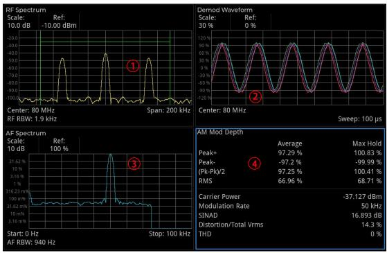
Figure 2-2 Amplitude Modulation Window
